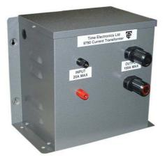
The 9790 is a heavy duty current transformer mounted in a steel case. It is suitable for use with Time Electronics 5025 and 5051 Multifunction Calibrators and the 5077 Power Calibrator. It extends the AC current capability to 100A rms. The maximum compliance voltage is approximately 0.3V at 100A. However in order to achieve this, very low resistance connecting leads must be used. Connection is via front mounted terminals.
